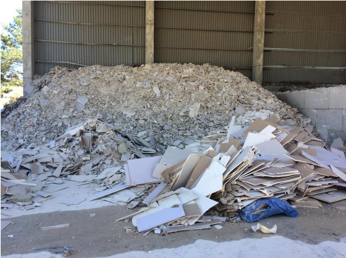
Figure 1: Sorted gypsum waste for recycling
