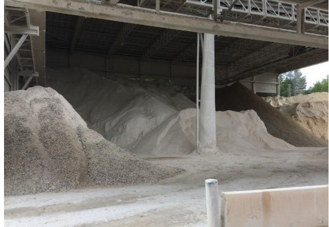
Figure 2. Intermediate storage of different fractions of crushed gypsum. On the left hand side of the picture, SRM is shown and PRM to the right.
